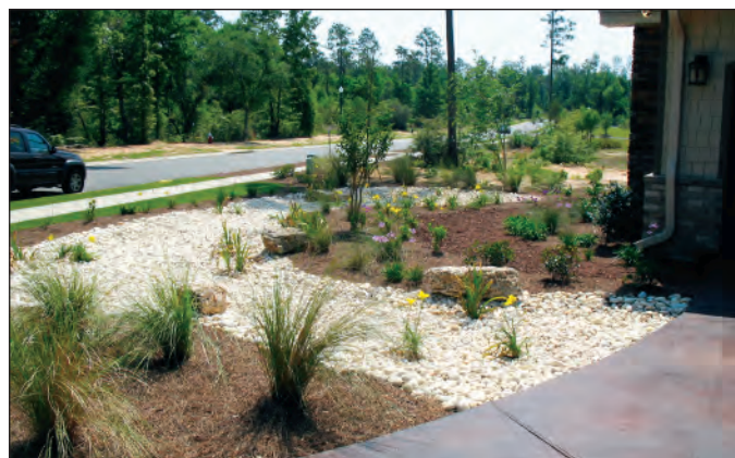
Rain gardens filter stormwater runoff before it soaks into the ground.
